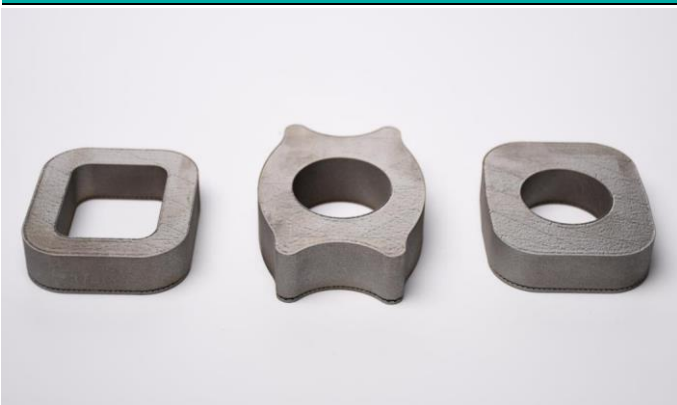
Figure 4 - Near-net shape watch cases produced by IPX
